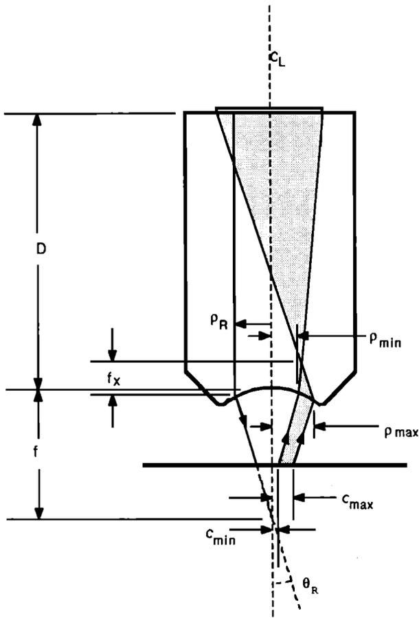
FIG. 2. Leaky ray bundle in the  $x$ - $z$  plane. The shaded region here represents the part of the leaky ray flux that excites the transducer. The total excitation flux is obtained by rotation about the lens axis.
