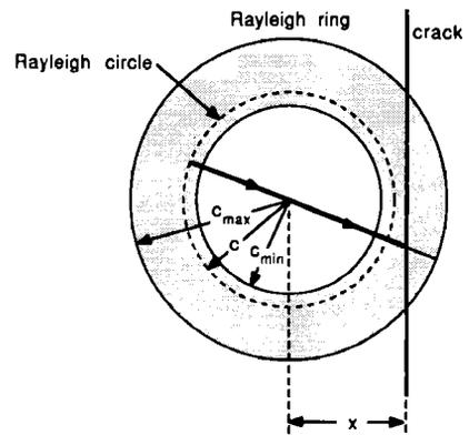
FIG. 3. A surface ray launched on the left that excites the transducer by leaking energy within the Rayleigh ring resulting in the leaky flux as shown in Fig. 2. As the ray crosses the crack the leaky field is reduced by the factor  $T$ .
