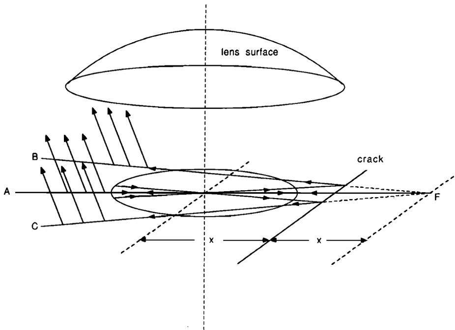
FIG. 4. Focusing and divergence of surface waves reflected from the crack. The circle on the surface is the Rayleigh circle of radius  $c = |z|\tan \theta_R$ .
