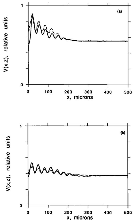
FIG. 5.  $V(x,z = z_0)$  for a lens having a circular aperture. The measured values are denoted by the solid line while the theoretical prediction is dashed: (a) is for  $z_0 = -300 \mu\text{m}$  and (b) is for  $z_0 = -400 \mu\text{m}$ .
