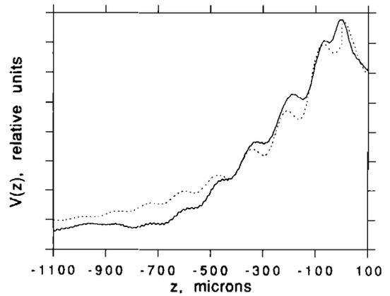
FIG. 3. Plot of  $V(z)$  of glass for a slot aperture lens: observed (solid) and calculated using the diffraction-corrected ray approach (dashed).
