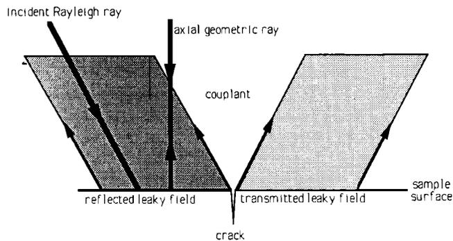
FIG. 6. Ray paths for the transducer voltage components  $V_G$ ,  $V_T$ , and  $V_{ref}$ . The component  $V_G$  results from the axial ray,  $V_{ref}$  from the reflected leaky field, and  $V_T$  from the transmitted leaky field.
