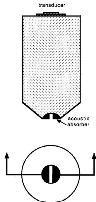
FIG. 1. Longitudinal cross section view of the slot lens. The transducer and lens rod have axial symmetry while the acoustic absorber blocks all but a slot-shaped area of the spherical lens surface.
