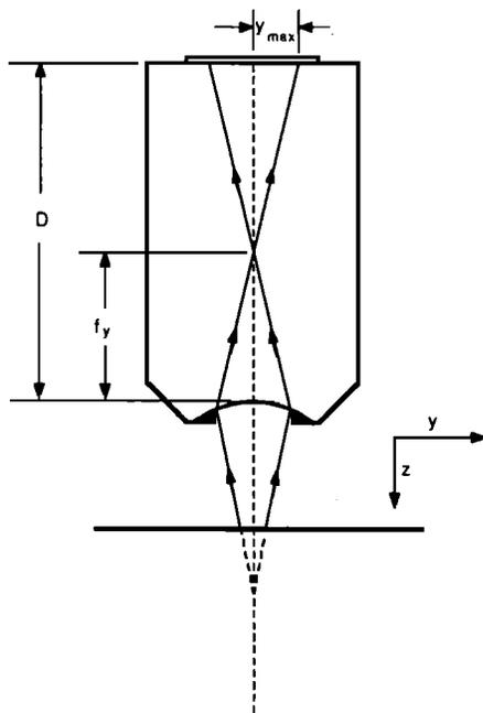
FIG. 12. Illumination of the transducer by a bundle of leaky rays that are reflected from the crack, shown in the  $y$ - $z$  plane.
