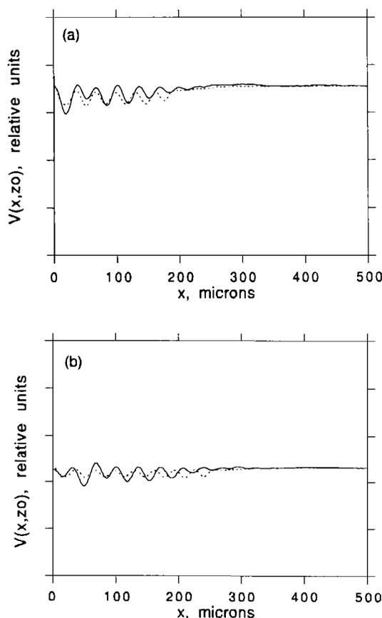
FIG. 13. Plot of  $V(x, z_0)$  for a slot aperture lens; observed (solid) and calculated (dotted): (a)  $z_0 = -346 \mu\text{m}$  and (b)  $z_0 = -474 \mu\text{m}$ .
