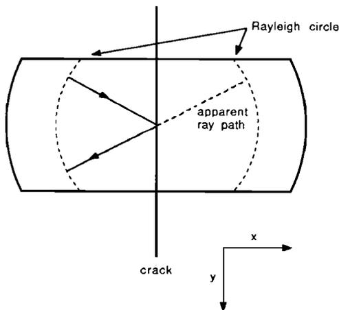
FIG. 14. Selected surface wave paths on the sample surface at  $z < 0$  containing a crack parallel to the  $y$  axis at  $x = 0$ .
