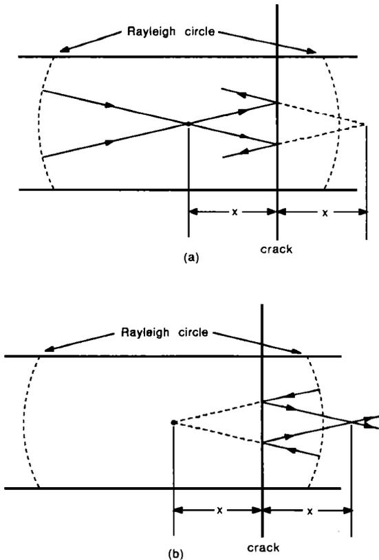
FIG. 11. Focusing of surface rays reflected from the crack on the (a) left and (b) right side of the Rayleigh circle.
