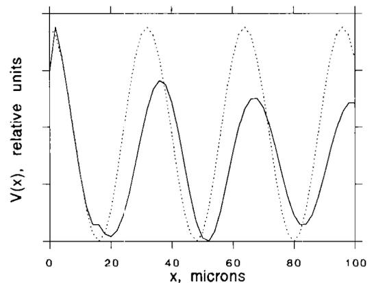
FIG. 15. Behavior in the vicinity of the crack: (a) calculated  $V(x, z_0 = -346 \mu\text{m})$  for the slot aperture lens (solid) and (b) the function  $\cos(2k_R x)$  (dashed).
