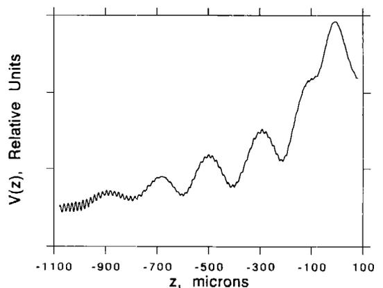
FIG. 4. Observed  $V(z)$  of  $y$ -cut quartz with slot oriented at  $90^\circ$  to the crystalline  $x$  axis.
