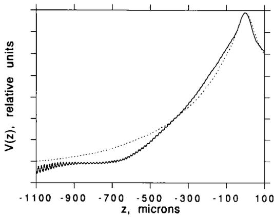
FIG. 2. Plot of  $V(z)$  of Teflon for a slot aperture lens: observed (solid) and calculated using the diffraction-corrected ray approach (dashed).
