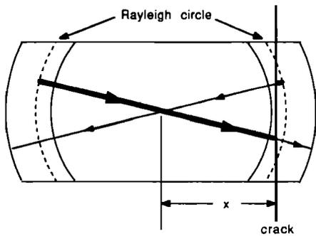
FIG. 8. Geometry of a surface ray that is excited on the left and leaks energy to the right of lens axis. After the ray crosses the crack the leaky field is reduced by the factor  $T$ . A left propagating ray is also shown.
