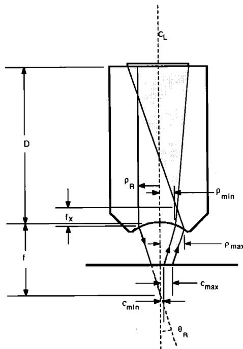
FIG. 7. Leaky ray bundle in the  $x$ - $z$  plane. The shaded region delineates those rays that ultimately excite the transducer. For clarity of the figure, only the ray perpendicular to the transducer is shown as exciting the surface wave.
