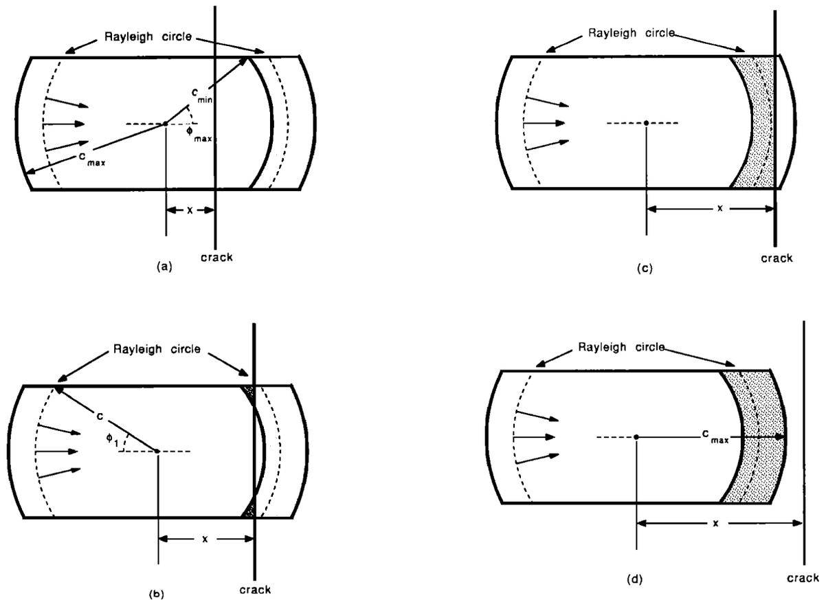
FIG. 9. Distinct ranges of crack displacement that lead to different geometric relations in determining  $Q_R$ : (a)  $0 < x < c_{\min} \cos \phi_{\max}$ , (b)  $c_{\min} \cos \phi_{\max} < x < c_{\min}$ , (c)  $c_{\min} < x < c_{\max}$ , (d)  $x > c_{\max}$ . The region of leaky radiation that reaches the transducer is shown as shaded, with the more dense shading indicating leaky radiation resulting from surface waves that are unscattered by the crack.
