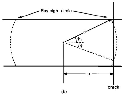
FIG. 10. Distinct ranges of crack displacement that lead to different geometric relations in determining  $Q_L$ : (a)  $0 < x < c \cos \phi_1$ , (b)  $c \cos \phi_1 < x < c$ , and (c)  $x > c$ .
