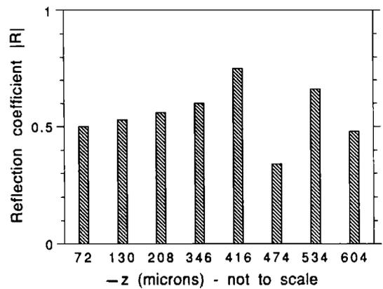
FIG. 16. Magnitude of surface wave reflection coefficient deduced from measurements made of a cracked glass sample using the slot lens.
