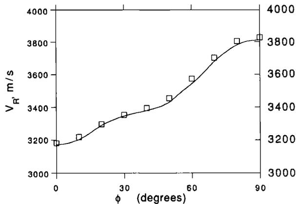
FIG. 5. Rayleigh wave velocity  $v_R$  of  $y$ -cut quartz as a function of direction of propagation angle  $\phi$  measured from the crystalline  $x$  axis: accepted (solid line) and measured values using the slot lens (open boxes).
